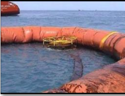
Figure 22: Skimmer positioned in boom apex (SINTEF)
