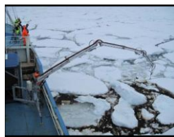
Figure 20: 2009 SINTEF JIP FEX testing the articulated spray arm (SINTEF)
