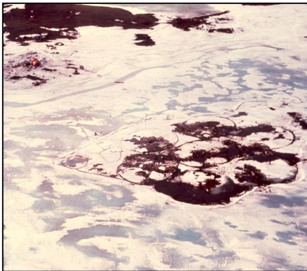
Figure 4: Oil appearance in melt pools during spring melt (Balaena Bay experimental spill 1974/75, Norcor/D.F. Dickins)
