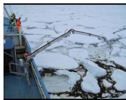
Figure 21: Photos taken during field tests of OMA-treated oil in ice after enhancing the dispersion with propeller wash of an ice breaker (SINTEF)
