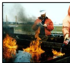
Figure 8: Tank testing to determine ignitability limits (SL Ross Environmental Research Limited)
