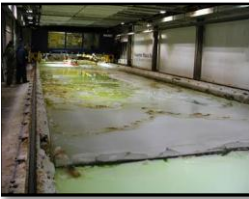
Figure 17: Tank testing in ice with dispersants. This picture is the Aker Arctic ice test basin and is relevant to the Spring et al. 2006 and Nedwed et al. 2007 work with icebreakers described below
