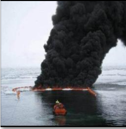
Figure 9: In-situ burning within drift ice using fire-resistant boom (SINTEF)
