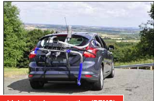
Light-duty in-use testing (PEMS)
