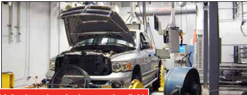
Light-duty chassis-dyno testing (lab)
