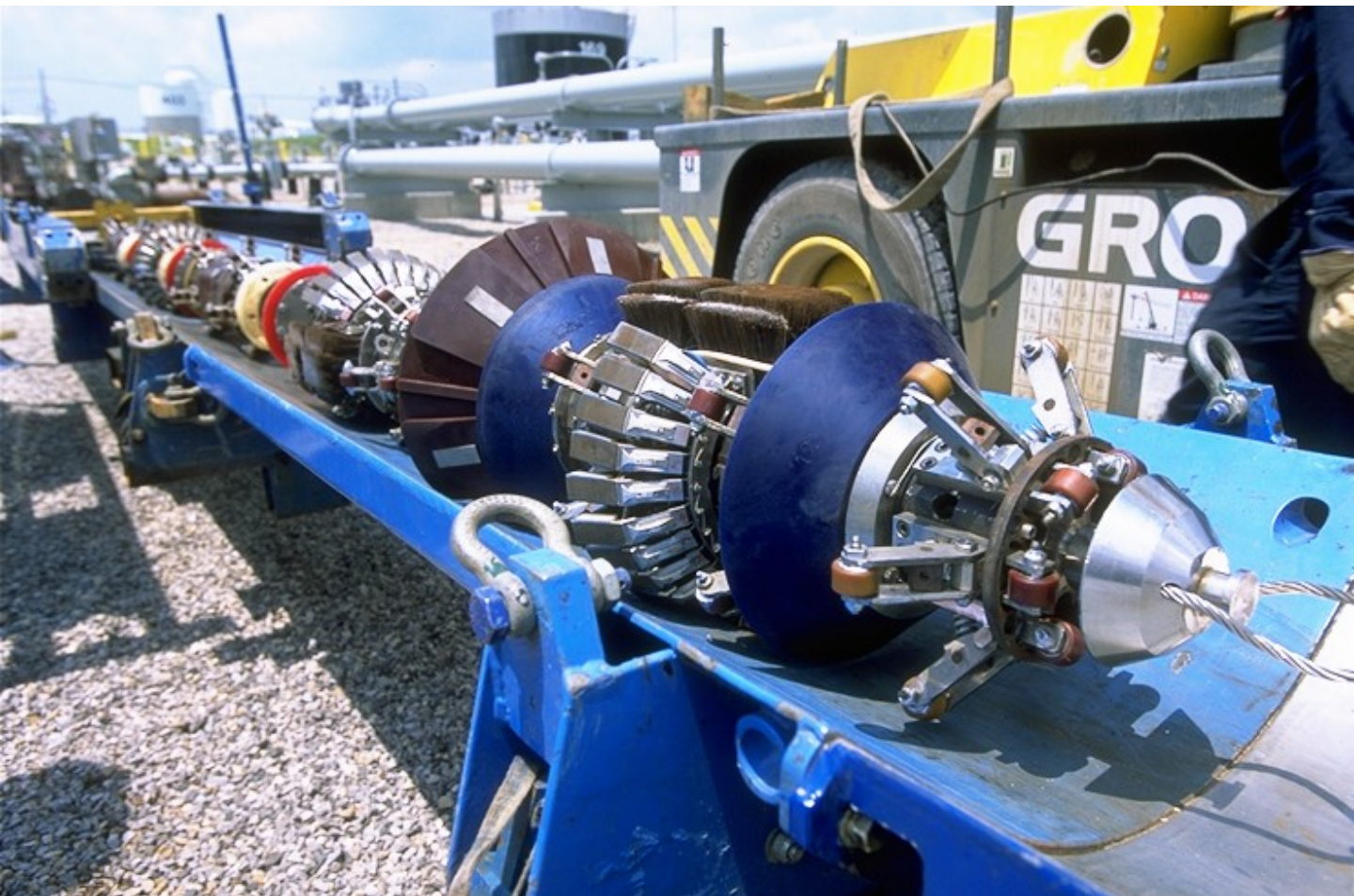
Pipeline operators use “smart pig” inspection devices that travel through pipelines analyzing and diagnosing issues in the pipeline.
