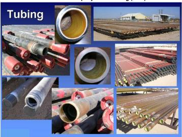
Figure 10 Glass Reinforced Epoxy Lined Tubing (GRE) <sup>9</sup>
