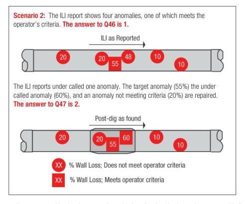
Again, all anomalies not covered by the sleeve are cleaned using abrasive blasting and are recoated before backfilling the ditch.
