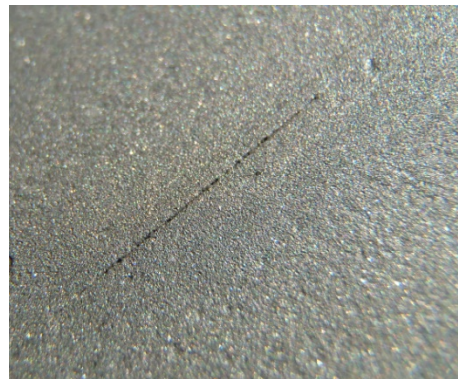
Figure 3: Visually Verified Bondline LOF (Courtesy of Riccardelli Consulting Services)
