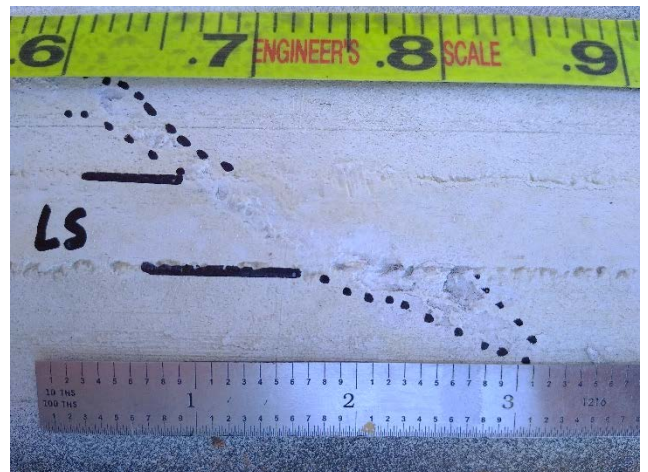
Figure 14 EML across ERW weld (Courtesy of Riccardelli Consulting Services)
