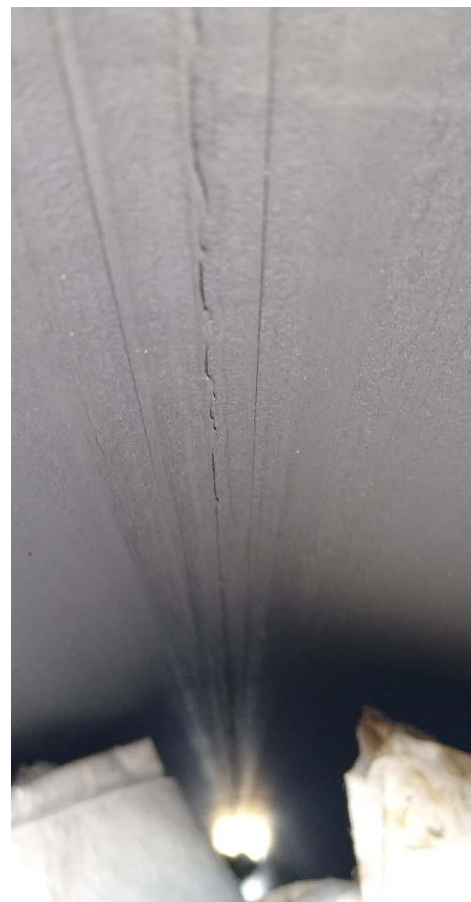
Figure 8: Under trim producing erratic ID protrusion. (Courtesy of Riccardelli Consulting Services)
