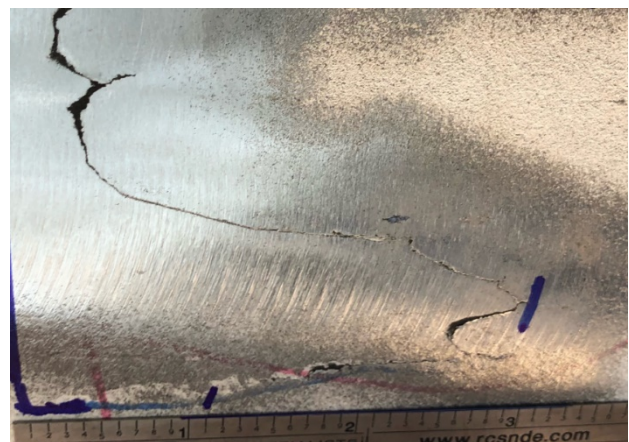
Figure 4: Surface breaking, sloping and oriented lamination (Courtesy of Riccardelli Consulting Services)
