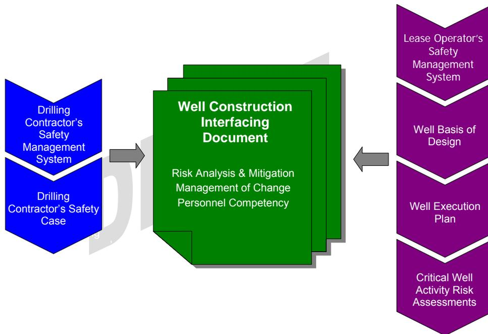
**The Well Construction Interfacing Document (WCID) addresses the management of well construction activities and mitigates unexpected events that impact HSE.**
