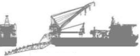
Pipelay vessel – rigid
