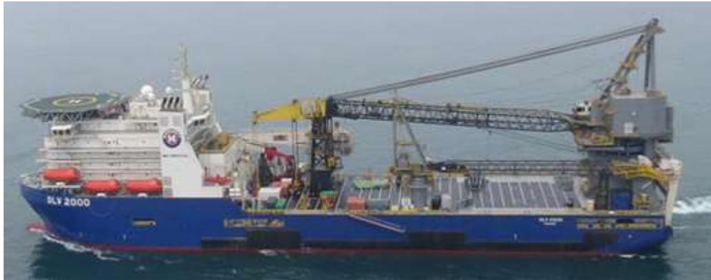
Figure 9 – Large conventional ship shape heavy lift vessel
