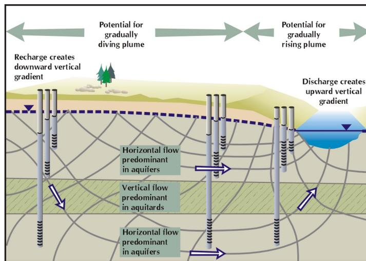
Figure 2. Expected groundwater flow conditions within a watershed
