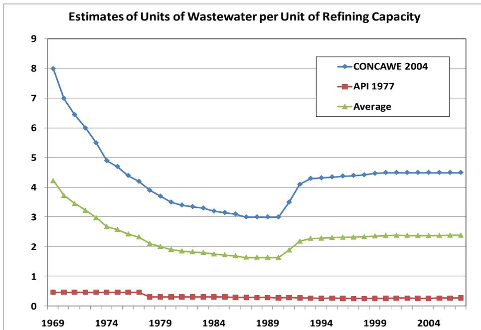
**Figure 41: Estimates of Units of Wastewater per Unit of Refining Capacity**
