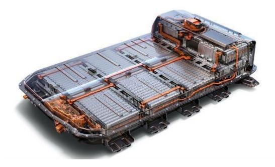
Figure 56 Chevrolet Bolt Battery Pack<sup>317</sup>
