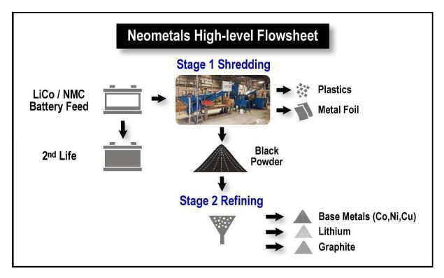
Figure 30 High-level Flow Sheet for Neometals Feed Preparation and Hydrometallurgical Processing Facilities (June, 2019)
