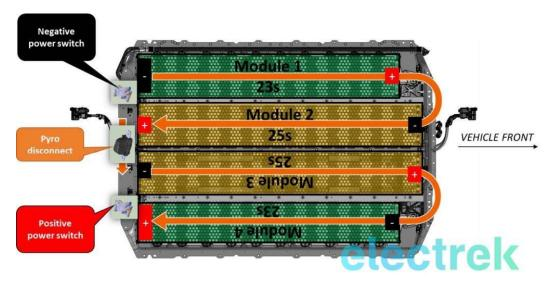
Figure 60 Distribution of Cells in a Tesla Model 3 Battery Pack<sup>325</sup>
