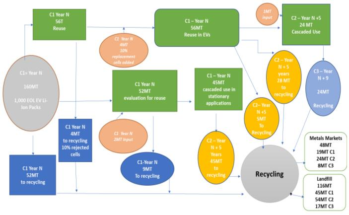
Figure 38 Material Flow Assumptions on Which Energy Analysis is Based (Adapted from Richa et al) <sup>187</sup>
