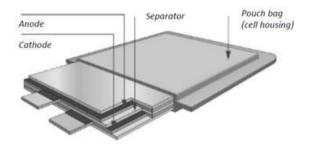
Figure 54 Li-ion Battery Cell – Pouch Design<sup>311</sup>
