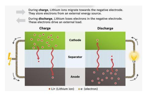
Figure 51 Schematic Showing How a Li-ion Battery Works<sup>299</sup>
