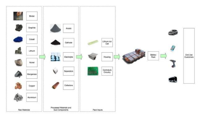
Figure 62 Li-ion Battery Supply Chain<sup>329</sup>
