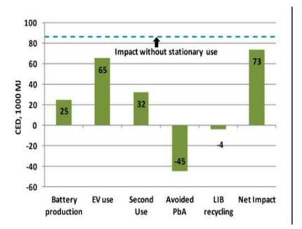
Figure 40 Estimated Comparative Energy Impacts of EV Battery Reuse <sup>191</sup>
