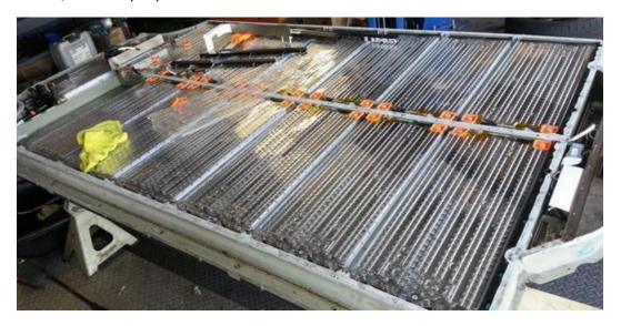
Figure 58 Photograph of a Tesla S Battery Pack<sup>321</sup>
