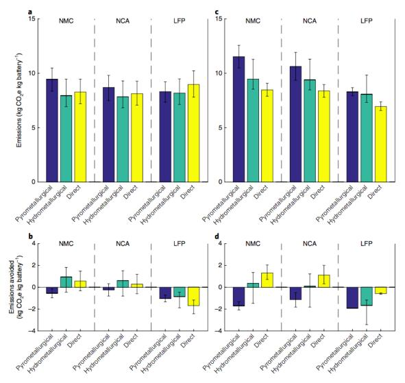
Figure 45 EV Battery Recycling Emissions from Different Recycling Processes for Cylindrical Cells (a,b) and Pouch Cells (c,d)<sup>203</sup>
