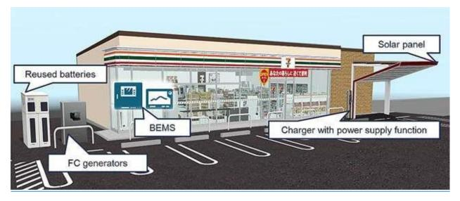
Figure 16 Reused EV Batteries Power a 7-Eleven Store in Japan
