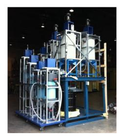
Figure 22 American Manganese Electrolytic Manganese Dioxide Recovery Pilot Plant (by Kemetco) for Low-Grade Manganese Ores
