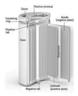
Figure 53 Li-ion Battery Cell - Cylindrical Design<sup>310</sup>
