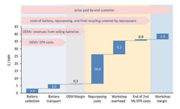
Figure 18 Cost Components for a Repurposed EV Battery in the EU in 2030
