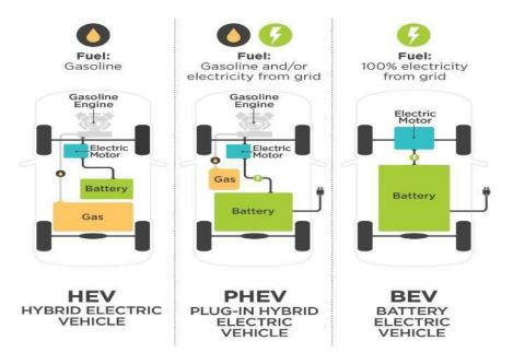
Figure 50 Schematic Showing Elements of HEV, PHEV and BEV<sup>289</sup>
