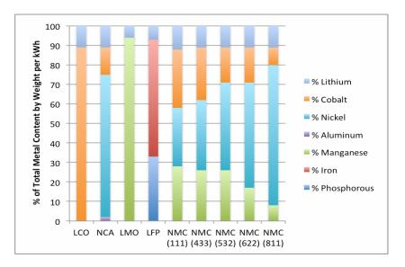
Figure 52 Metal Content of Li-ion Batteries by Cathode Chemistry, % of Total Metal Content by Weight by kWh<sup>306</sup>
