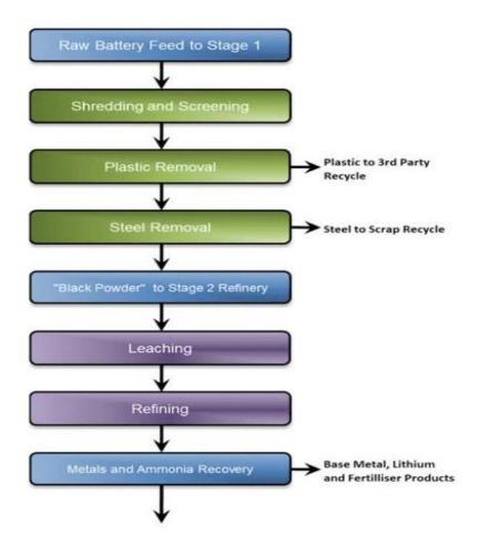
Figure 27 Neometals Process Flow Chart For Proposed Plant
