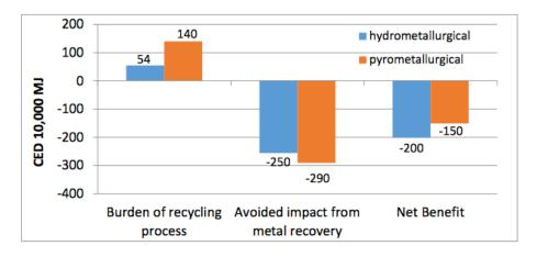
Figure 44 Net Energy Benefit of EV Battery Recycling (CED)<sup>199</sup>
