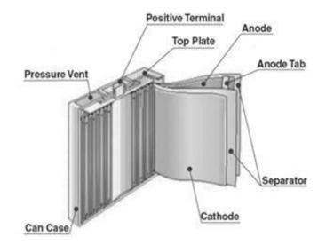
Figure 55 Li-ion Battery Cell – Prismatic Design<sup>312</sup>
