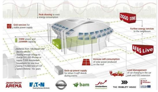
Figure 72 Nissan EV Batteries Used in Back-Up Power System at Amsterdam Johann Cruyff Arena
