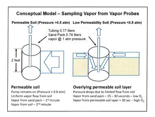
Slide 7 - McAlary, et al. (2009) presents model for sampling vapor from low permeable soil where pressure in sand pack is reduced by removal of vapor during sample collection. With time, vapor will be replenished into sand pack by 'advective' flow due to pressure gradient developed between sand pack and surrounding soil.
