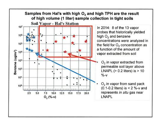
Slide 8 - The 1 liter samples previously collected at Hal's contained a mixture of 'low  $O_2$ /high benzene' vapor from sand pack and 'high  $O_2$ ' vapor from permeable soil overlying LNAPL
