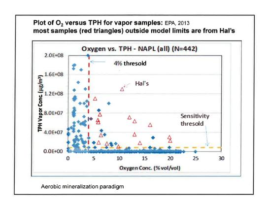
Slide 4 - Measurements with  $O_2$  < 4 % or TPHV < 10,000 ug/m³ are considered consistent with diffusion/biodegradation model. Most samples falling outside limits for the model are soil vapor samples taken at Hal's site, Green River Utah.
