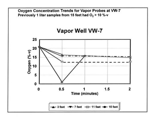
Slide 6 - At depths 3, 7, and 11 feet:  $O_2$  initially decreased (remove air from tube) – then remained relatively constant for 2 minutes.
