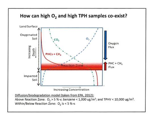
Slide 3 - Conceptual model used to evaluate potential PVI risk. Based on model, high concentrations of benzene and oxygen can only exist within a narrow depth range above the source of TPH vapor.
