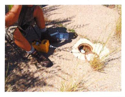
Slide 5 - The approach used to address Objective 1 was to continually monitor gas composition ( ${\rm O_2/CO_2}$ ) of vapor extracted from soil so that any change in the composition of vapor would be documented. An Eagle field meter was connected to individual vapor probes and soil vapor was extracted at a rate of 1 L/min (or less). The pump on the instrument is set to stop when pressure was reduced to 0.8 atmospheres pressure in tubing (sand pack).
