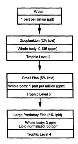
Figure 2-9. Food chain biomagnification of a typical PCB ( $K_{ow} = 10^6$ ). The BAF, based on lipid in the tropic level 4 predator, is 6.0 x 10<sup>7</sup>. Note that trophic level 1 (phytoplankton) is not included in this example.
