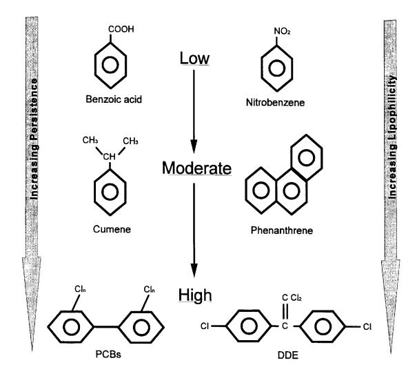
Figure 2-5. Chemical structures of selected organic compounds having increasing environmental persistence and lipophilicity. Note that high environmental persistence does not always lead to large BAFs.
