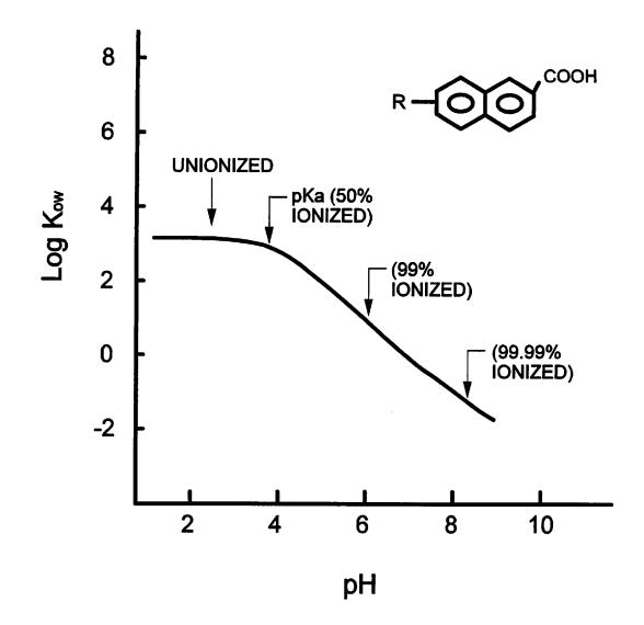
Figure 2-4. The effects of pH on the K<sub>ow</sub> or the lipophilicity of a weak organic acid, where R is an alkyl group (modified from Connell, 1990). The pH at which a compound is half ionized and half unionized is denoted pKa.
