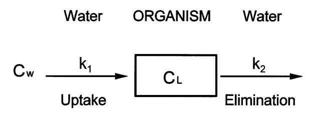
Figure 2-8. Single-compartment model for the uptake and elimination of lipophilic chemicals by an organism, where  $C_W$  is chemical concentration in water,  $C_L$  is chemical concentration in the organism's lipid, and  $k_1$  and  $k_2$  are rate constants.
