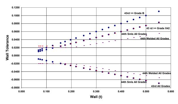
b For pipe with D >= 355,6 mm (14.000 in) and t >= 25,0 mm (0.984 in), the wall-thickness tolerance locally may exceed the plus tolerance for wall thickness by an additional 0,05 t, provided that the plus tolerance for mass (see 9.14) is not exceeded.
